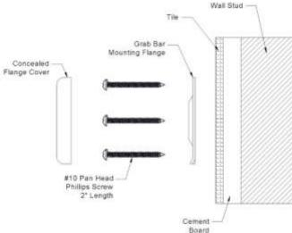
Apply a bead of silicone around the Grab Bar Mounting Flanges on the mounting surface to ensure a water-tight seal will be created at all mounting locations. Secure the grab bar to the wall using six (6) #10 Pan Head Phillips sheet metal screws (provided) and screw into the 1/8" holes created in the solid wood backing. Complete the grab bar installation by covering the mounting flanges with the Concealed Flange Covers, snapping them into place.
